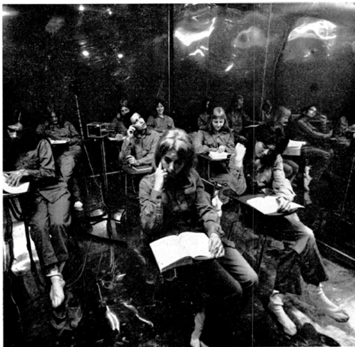
FIG. 5. Subjects wearing a standard uniform (0.6 clo) during thermal studies in the environmental test chamber at the Technical University of Denmark. During the studies, physical and physiological measurements are correlated with the subjective evaluations of the subjects.
